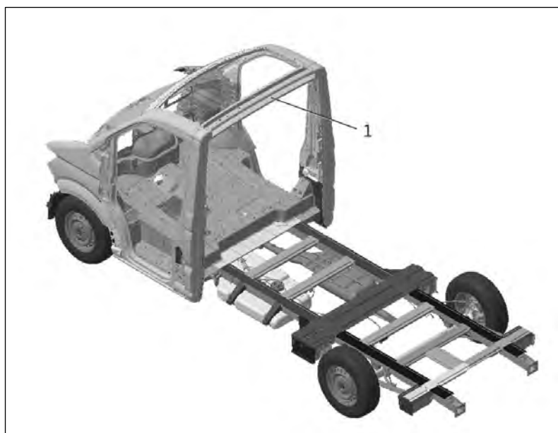
Fig. 1: Cowl panel with flat frame chassis (K4Z) / 1-auxiliary roof cross strut for transport
