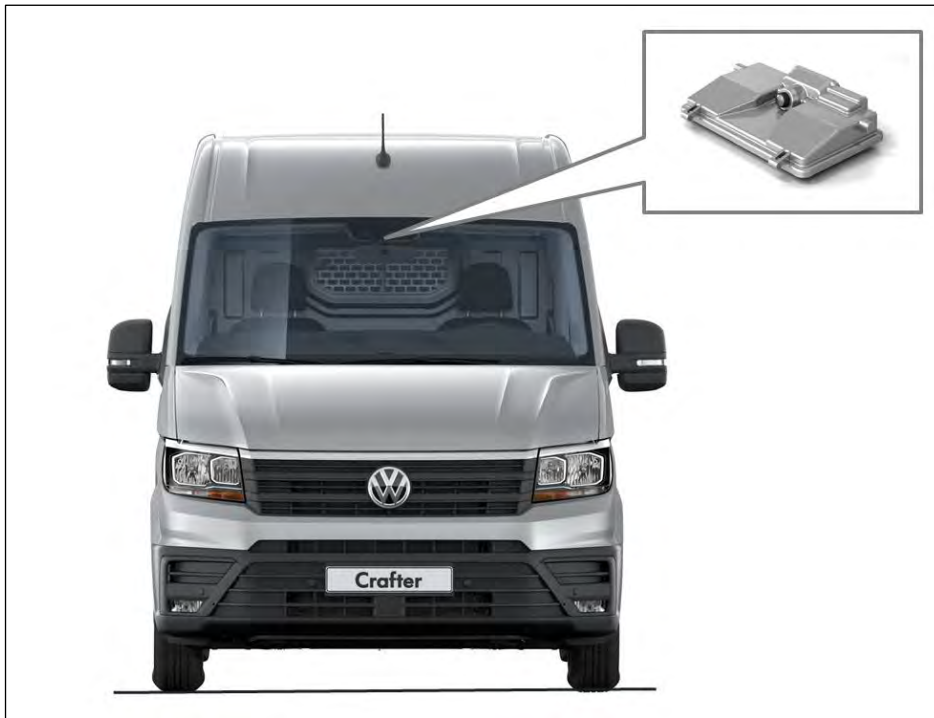
Fig. 1: Position of front camera for driver assist systems in vehicle
