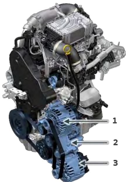
Power take-off system with additional alternator
