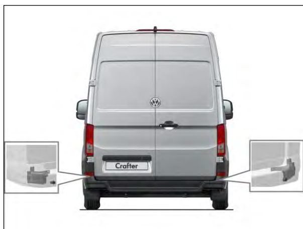
Fig. 3: Position of the radar sensors behind the bumper cover on the left and right
