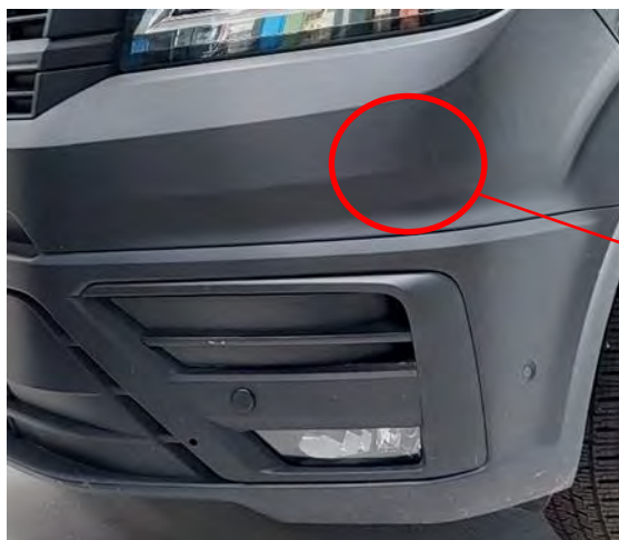
Fig. 3: Position of the radar sensors behind the front bumper cover
