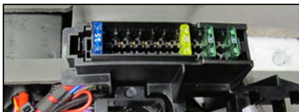
Detail A: Fuse holder – Connection point for second battery
