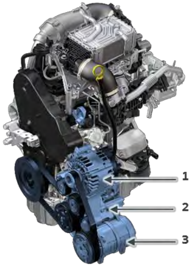
Power take-off system with additional air conditioner compressor
